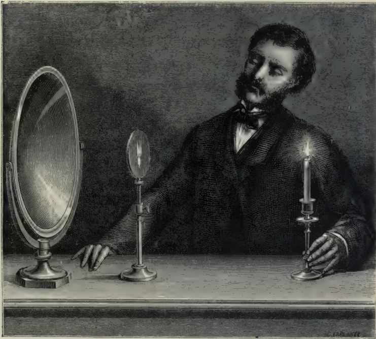
FIG. 51. —Formation of Image of Candle by Reflection.
